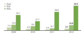
Concentrations of Air Pollutants from Boilers at the Hungary Plant (Unit: mg/L)
